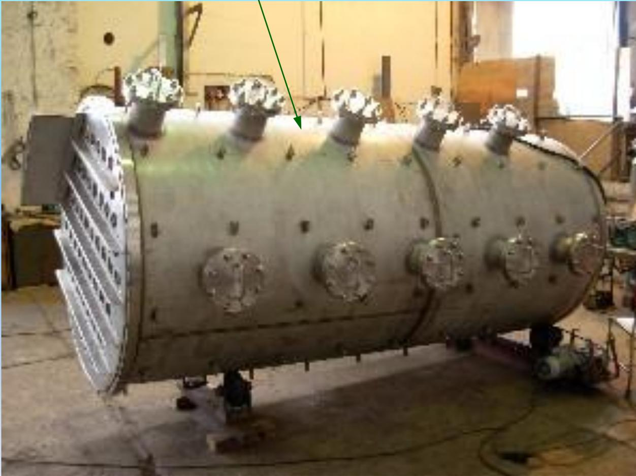
**A chemical reactor with heat exchanger**
