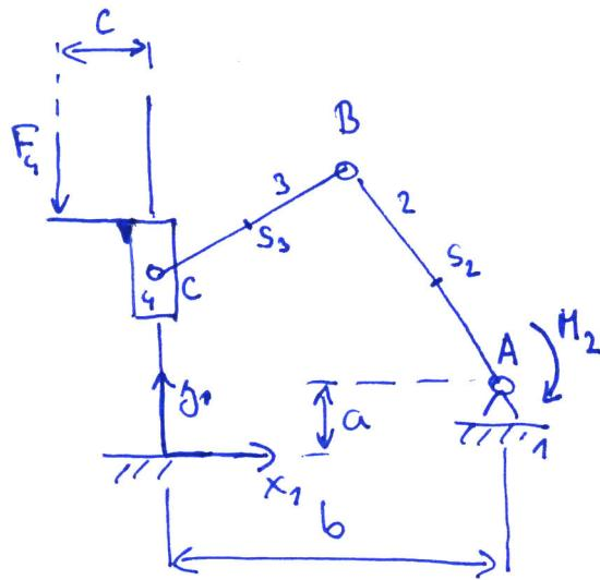
$$n = 3 \cdot (4-1) - 3_{\text{rot}} \cdot 2 - 1_{\text{pos}} \cdot 2 = 9 - 6 - 2 = 1^{\circ} \text{ vlnost}$$
