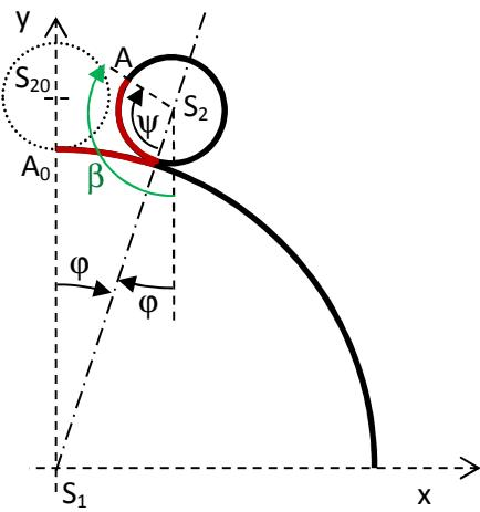
$$ma_t = m(R + r)\ddot{\varphi} = G \cdot \sin\varphi - T_0$$
