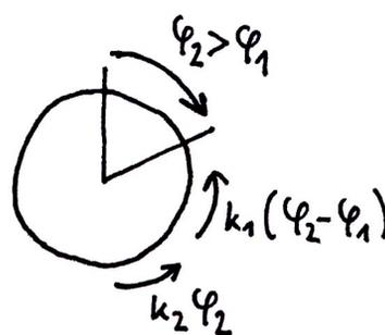
$$I_1 \ddot{\varphi}_1 = M_1(t) + k_1(\varphi_2 - \varphi_1) \rightarrow I_1 \ddot{\varphi}_1 + k_1 \varphi_1 - k_1 \varphi_2 = M_1(t)$$
