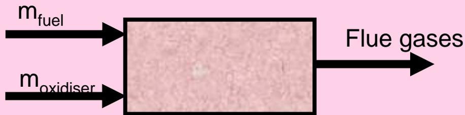
Calculation of fuel and oxidiser consumption is the most difficult part. Mixture fraction method is the way, how to avoid it
