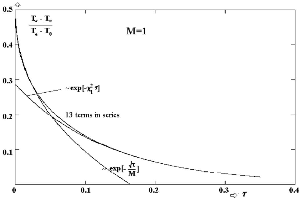
Fig.2 Dimensionless temperature of wall as a function of  $at/R^2$  for  $M=1$ . Curves represent the short time solution Eq.(28), and the series (27) for 13 terms or just 1 term.
