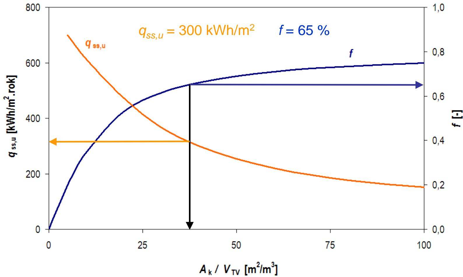
increase of solar fraction means decrease of specific heat gain
