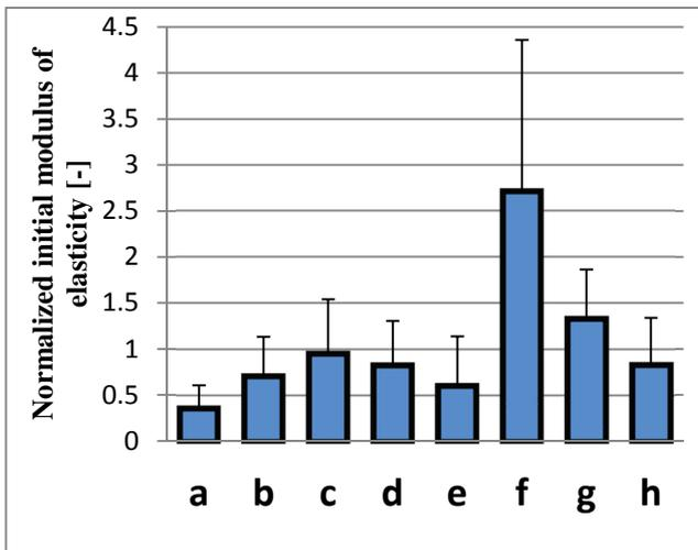
Fig. 4 Normalized initial moduli of elasticity. The figure shows how many times the one group of samples is stiffer than the average. The horizontal tick above each bar represents standard deviation.
