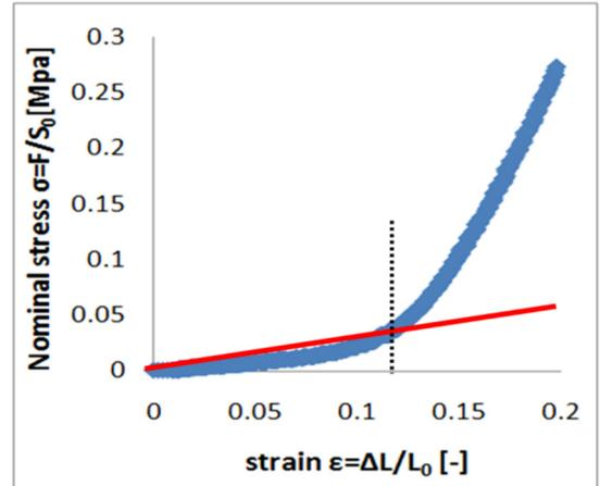
Fig. 3 Example of stress-strain relationship. The slope of red line represents initial secant modulus of elasticity.
