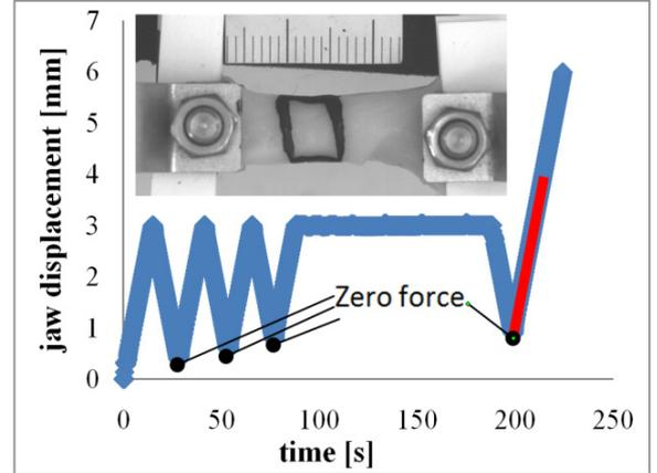
Fig. 2 Loading regime consists in four precycles (up to  $\lambda=1.1$ ), 100s stress relaxation and final loading cycle up to a failure. Red line denotes evaluated zone. The picture of clamped sample is inserted.
