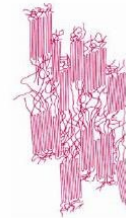
4. Separation of crystalline block segments during the third stage
