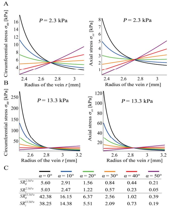
Fig. 3 The simulation of the influence of opening angle  $\alpha$ . The circumferential and axial stress gradients through the vein wall for transmural pressure 2.3 kPa (panel A) and for 13.3 kPa (panel B). Stress ratios at the inner and outer radius quantifying the stress gradient (panel C)
