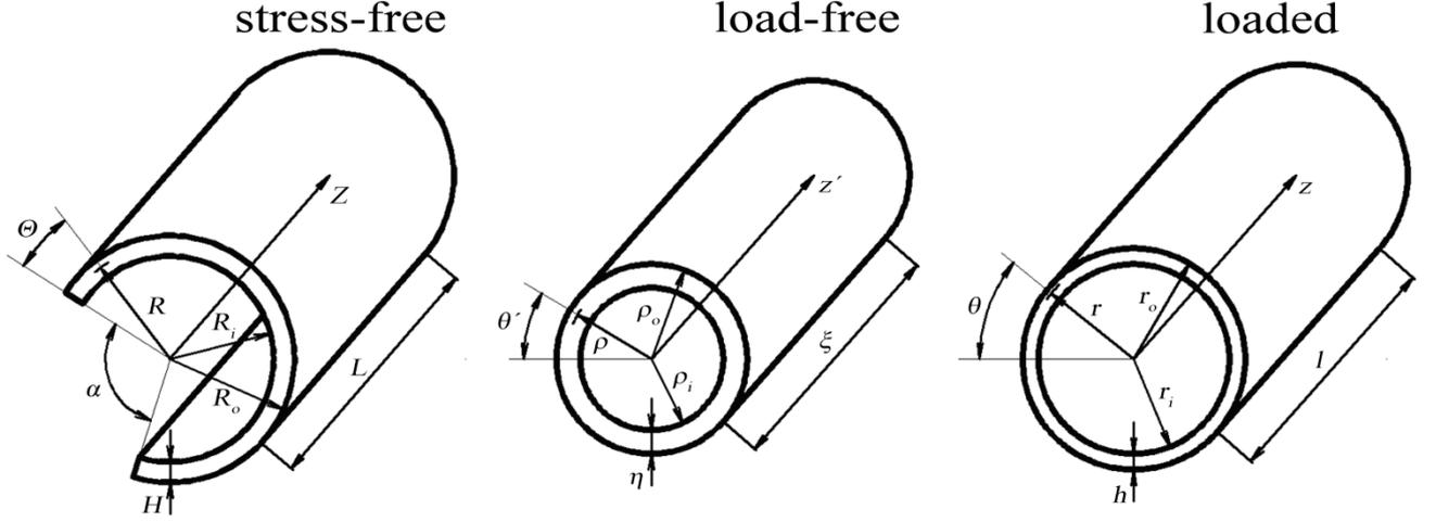
Fig. 1 Kinematics of the deformation with opening angle taken into account
