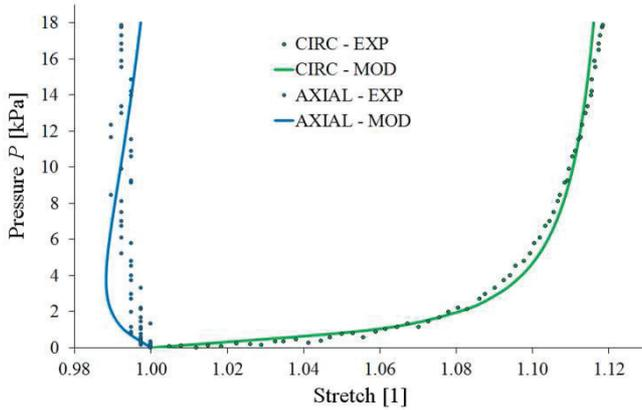
Fig. 2 Experimental (points) and model (solid line) pressure – stretch data for circumferential (CIRC) and axial (AXIAL) direction.
