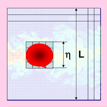
In order to resolve all details of turbulent structures it is necessary to use mesh with grid size less than the size of the smallest (Kolmgorov) eddies. N-grid points in one direction should be
