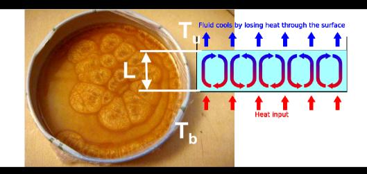
Even if the stability limit was exceeded the flow pattern is steady and remains laminar. At this stage the nonlinear convective term is not so important. Only if Ra<sub>1</sub> > 10<sup>9</sup> (approximately) eddies start to be chaotic, velocity fluctuates and the flow is turbulent.
