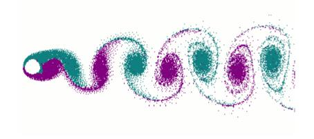
Even if the stability limit was exceeded the flow pattern is steady and remains laminar.
