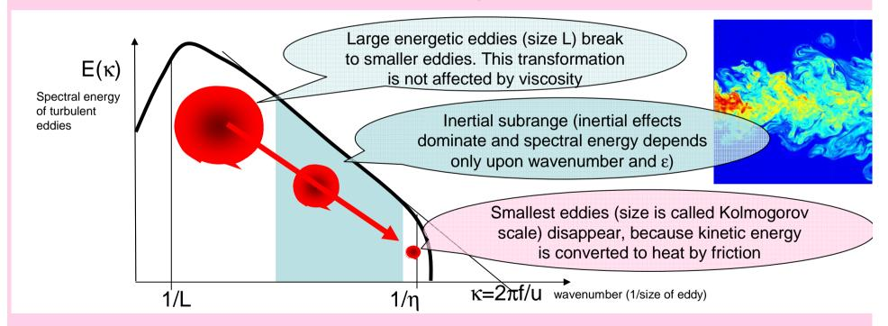
Typical values of frequency f~10 kHz, Kolmogorov scale  $\eta$ ~0.01 up to 0.1 mm Kolmogorov scale  $\eta$  decreases with the increasing Re
