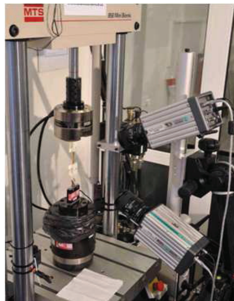
Figure 3. MTS Mini Bionix extensiometer and Q450 digital image correlation system
