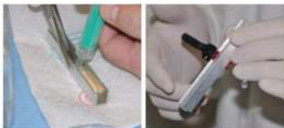
Figure 2. Bonding and pressing of vascular tissue strips by clips
