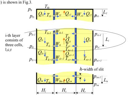
Geometry of two lateral channels (denoted by indices l,r) and central channel (c) is shown in Fig.3.
