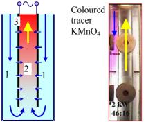
Figure 1. Continuous ohmic heater (scheme and photograph showing asymmetry of *flows*). 1-lateral channels;2-central channel,3-electrodes.
