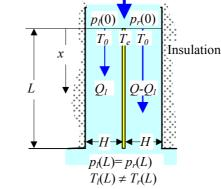
Figure 2. Parallel flows heated by wall at constant temperature  $T_e$ .
