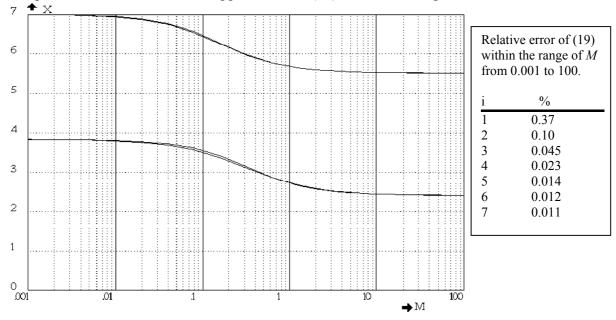
Fig.1 Eigenvalues  $\chi_1$  and  $\chi_2$  as a function of *M*, according to exact solution of Eq.(18) and approximation Eq.(19), which predicts slightly higher values within the range M $\in$  (0.01 – 1).
