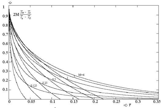
Fig.3 Time courses of  $2MT^*$  for M=0.125, 0.25, 0.5, 1, 2 and 4. Curves represent the short time solution Eq.(28), and series (27) were calculated with 20 terms using approximation Eq.(19).
