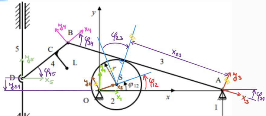
$$\underline{T}_{13} = \underline{T}_x(\overline{OA}) \cdot \underline{T}_\varphi(-\varphi_{31})$$
