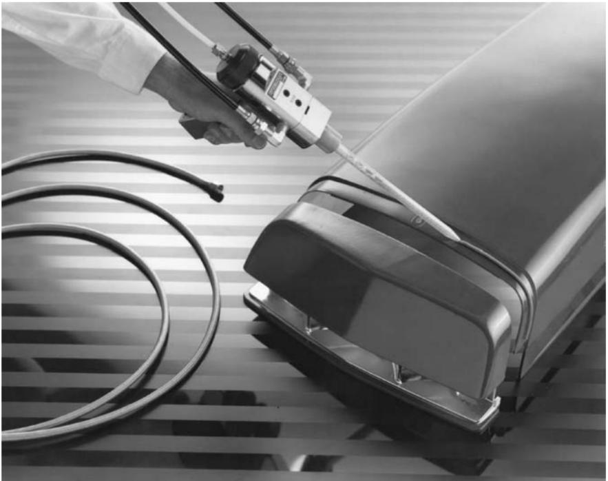
**Figure 18.7** Structural bonding of air intake on a tractor. Adhesive is metered and mixed in an on-line static mixing nozzle. (Photo courtesy of Sealant Equipment and Engineering, Inc.)
