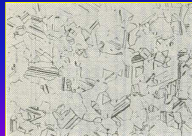
Annealed nickel silver alloy (65%Cu-10%Ni-25%Zn) structure of \alpha grains with twin bands
