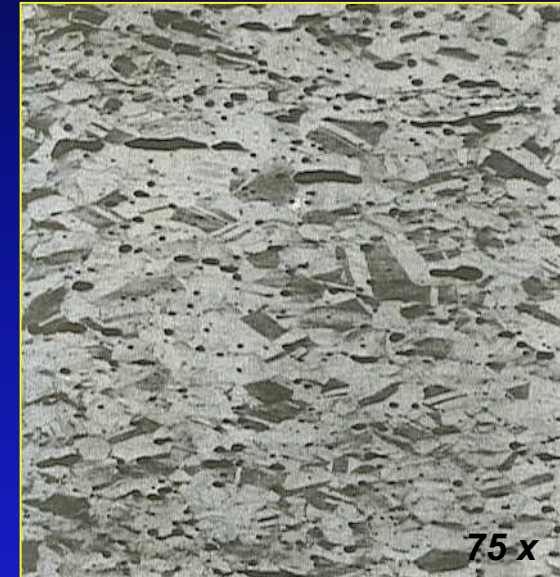
Free-cutting brass extruded rod showing elongated lead globules with the remained \alpha phase
