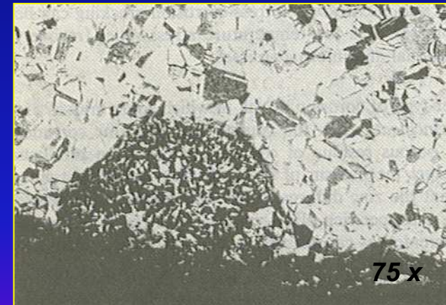
Dezincification of cartridge brass (70%Cu-30%Zn)
